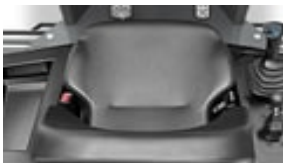
Seat contact control switch: If the driver leaves the driver's seat, the engine reduces speed to full stop.
