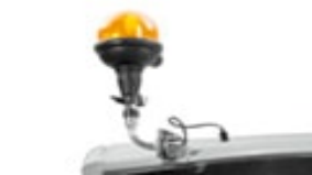
A rotating beacon enhances the vehicle's visibility.
