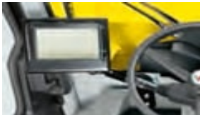
A camera and display minimize the blind spot in front of the vehicle, thus ensuring even more safety.
