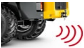
Back-up alarm: an acoustic alarm signals when the drive is in reverse gear.
